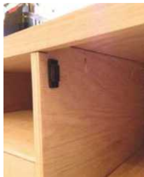
STEP 26. Add mirror tacks for additional holding of the plexiglass, then install the knobs
